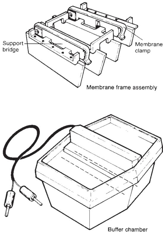
**Figure 2.5** An electrophoresis system. A membrane frame assembly and buffer chamber for the Gelman Sepra Tek electrophoresis system.
