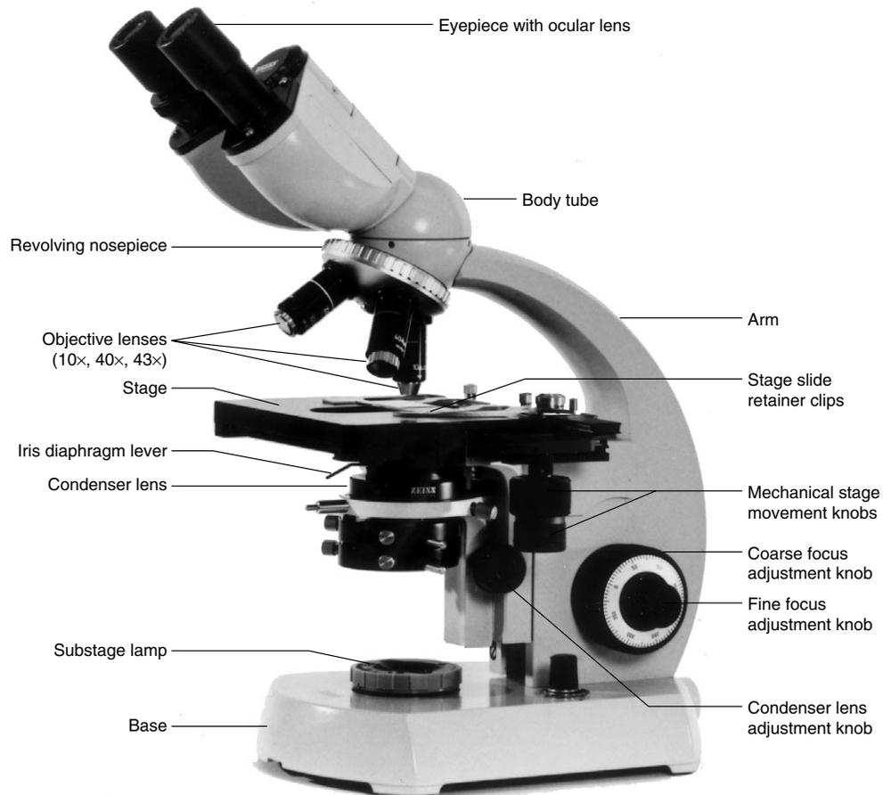
**Figure 1.1** The parts of a compound microscope.
