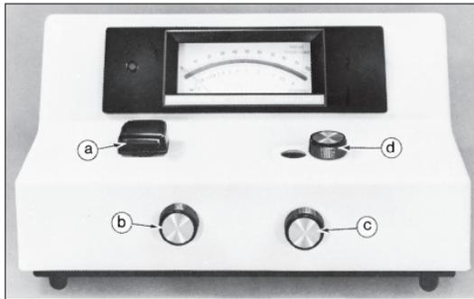
**Figure 2.2** A typical colorimeter (spectrophotometer).
