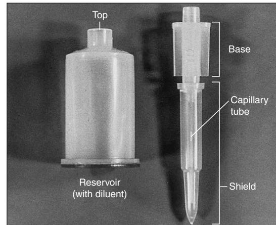
**Figure 6.2** The Unopette system (Becton-Dickinson). This consists of a reservoir containing the premeasured amount of diluent (left) and a plastic capillary tube within a shield (right) for puncturing the reservoir top and delivering a measured amount of whole blood to the reservoir.
