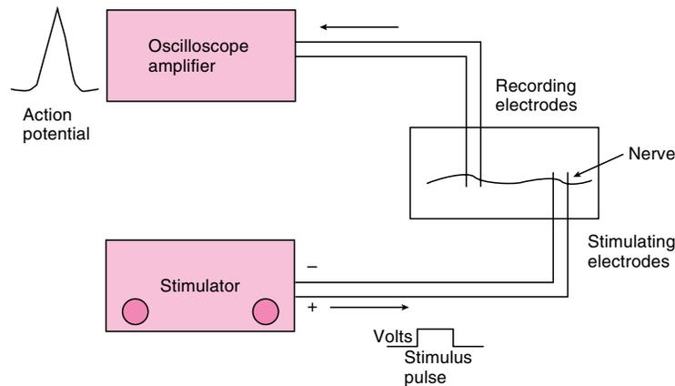
**Figure 3.5** Setup for recording from an isolated nerve. A nerve is laid across a pair of stimulating electrodes and a pair of recording electrodes. A stimulator delivers a square-wave pulse of a given voltage and duration to the nerve via the stimulating electrodes. This can be seen at the recording electrodes as the stimulus artifact (not shown). The action potential observed after the stimulus artifact represents the response of the nerve to the stimulus.
